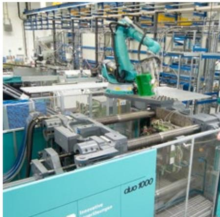
BITO bins and containers are produced in one of the most modern plants of the industry on high performance injection moulding machines with a clamping force of up to 27000 kN. In our finishing centre, a wide variety of bins and containers can be adapted to customer-specific requirements. The entire manufacturing process combines high levels of automation with utmost versatility.
