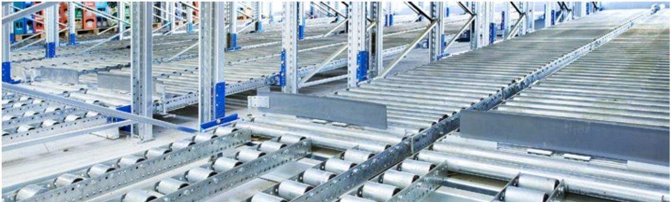
The BITO FlowStop load separator has been designed to reliably separate the first pallet at the picking face from the other pallets in the lane. This allows to retrieve the pallet at the picking face safely without lane pressure and without damaging the FlowStop load separator. The load separator has been fitted out of reach for truck forks. This means substantially lower repair costs as well as safe and convenient pallet loading and unloading.
