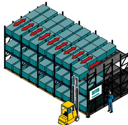
Operates according to the LIFO principle: last in, first out
