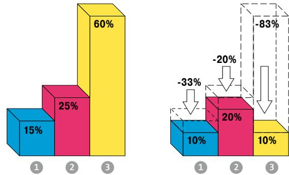
The optimum ergonomic layout of the picking area in front of an automated bin or tray storage installation reduces reading and picking times. There is almost no walking required for order pickers which reduces travel times considerably.
