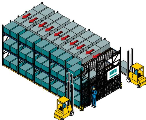
Operates according to the FIFO principle: first in, first out
