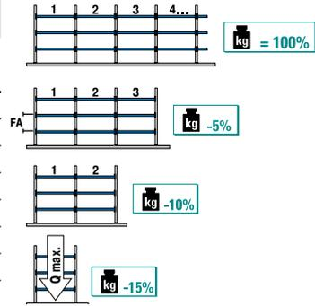
All values refer to a bay width of 2700 mm and racking rows of at least 4 bays. Shorter racking rows have a lower load capacity (cf. drawing on the right); the same applies to 3600 mm wide bays (please ask our team!). The bay load capacity table is only valid for bays with at least 2 beam levels and uniformly distributed shelf loads and bay loads.
