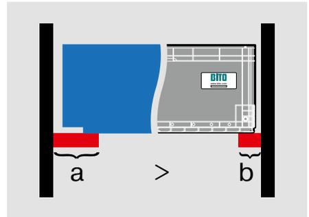
A wider base than is usual for European standard size stacking containers (389 mm instead of 363 mm) allows cutting down on the steelwork cost of AS/RS facilities.
