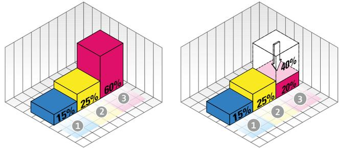
Compared to conventional pallet racking, pallet live storage reduces travel times by two thirds.
