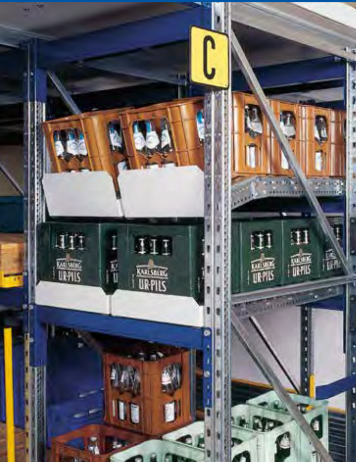
Lanes with front incline are ideal for single bottle picking, whereas straight lanes are preferred for beverage case picking
