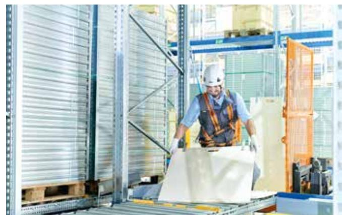
4. Push the intermediate board up to the yellow divider rail of the load separator.
