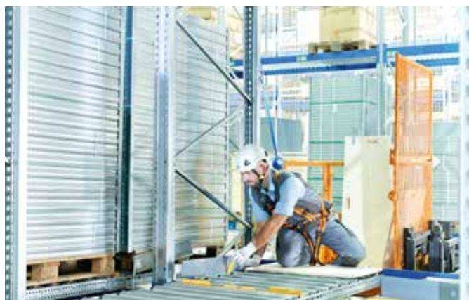
3. Swing activator of the FlowStop load separator to the side and secure it with the holding device.
