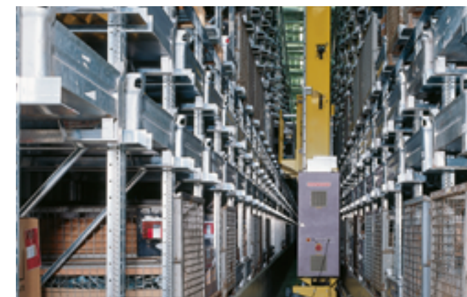
Automated pallet live storage facility with single position storage
