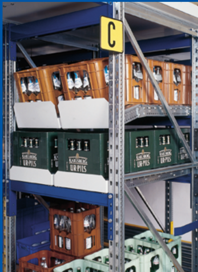
Lanes with front incline are ideal for single bottle picking, whereas straight lanes are preferred for beverage case picking
