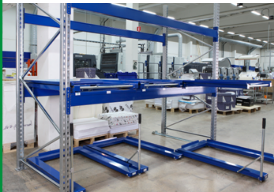
Pull-out pallet positions at floor level height and on the first beam level
