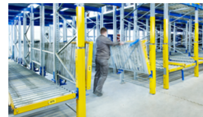
Tiltable/hinge-up roller conveyor segment
