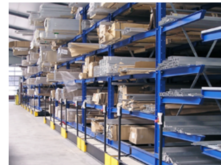
Mobile cantilever racking storing long loads
