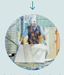
**4.** Lay the intermediate board against the yellow load separator stop bar.
