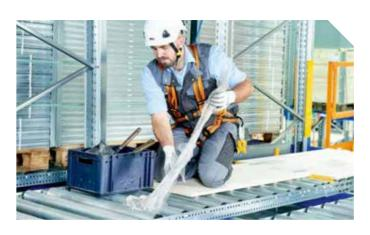
Removing dust, dirt, liquids and other impurities as well as foreign objects (e.g. packaging film) is just as easy with the PLS Access Kit. The place to be cleaned can be conveniently reached walking on the access boards.
