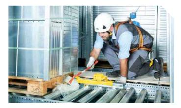
Access the trouble spot via the adjacent lane that has been covered by slip-proof boards. Use the pallet blocking device to prevent trouble pallets from moving down the lane unexpectedly. Properly secured by the access kit the assembly person can walk into the lane to find out what caused the problem and to fix it.
