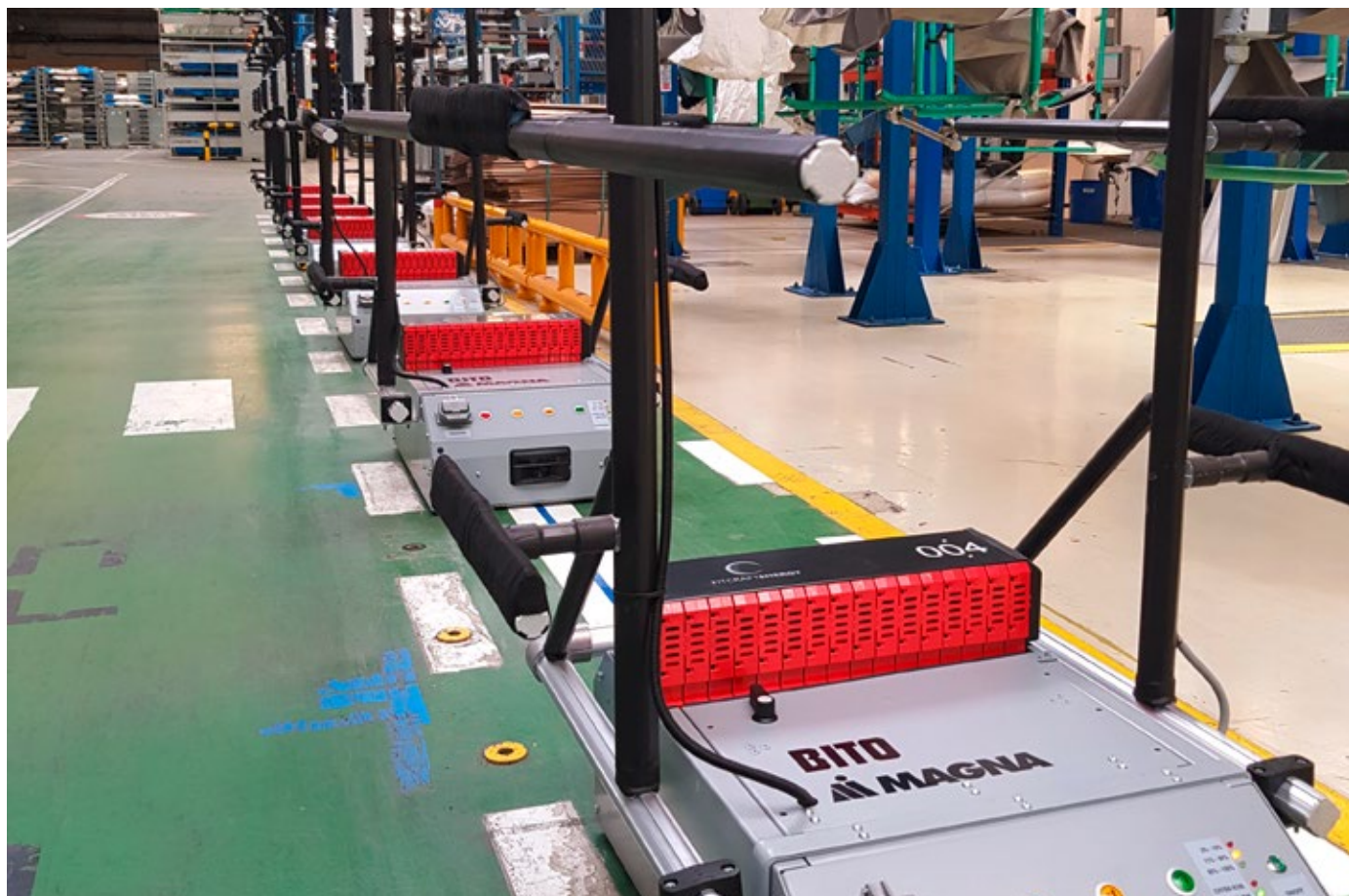
LEO custom with application specific on-top frame for transporting plastic car parts
