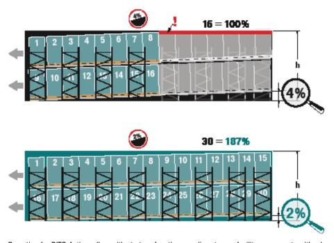
By opting for BITO Active rollers with start-up function your live storage facility can operate with a lane incline as low as 2%.
