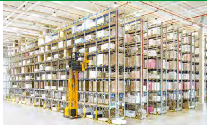
High-bay pallet racking
