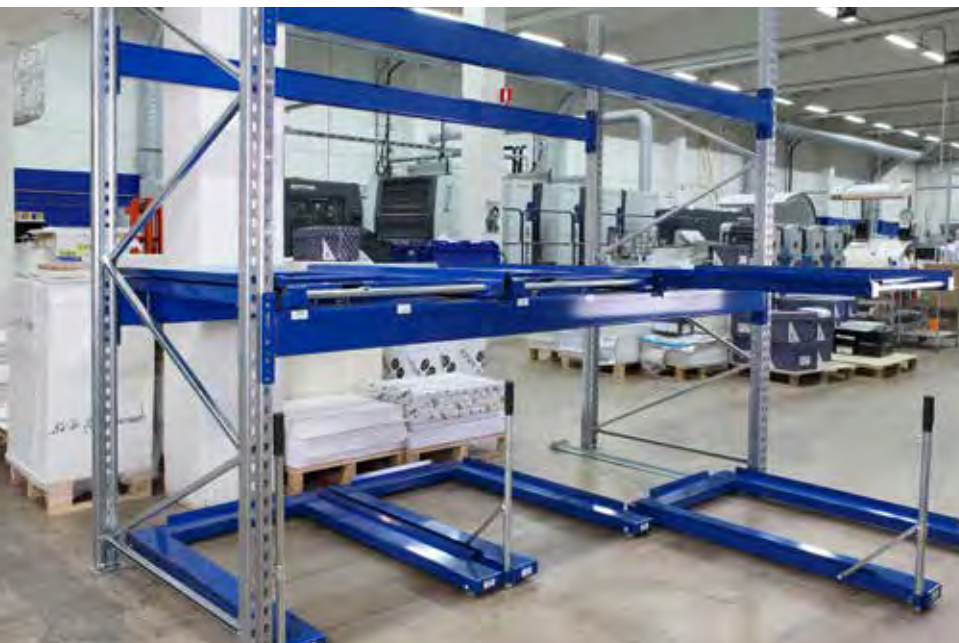
Pull-out pallet positions at floor level height and on the first beam level
