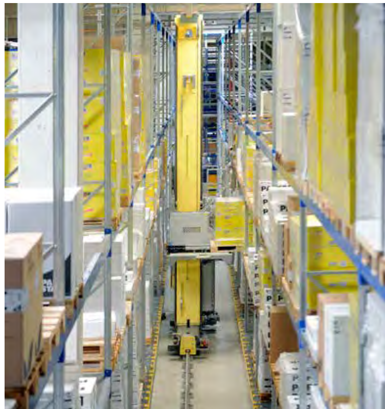
Papstar, static pallet storage on the upper levels, while pallets that are fed into the live storage floor level move down the lanes to the picking face.
