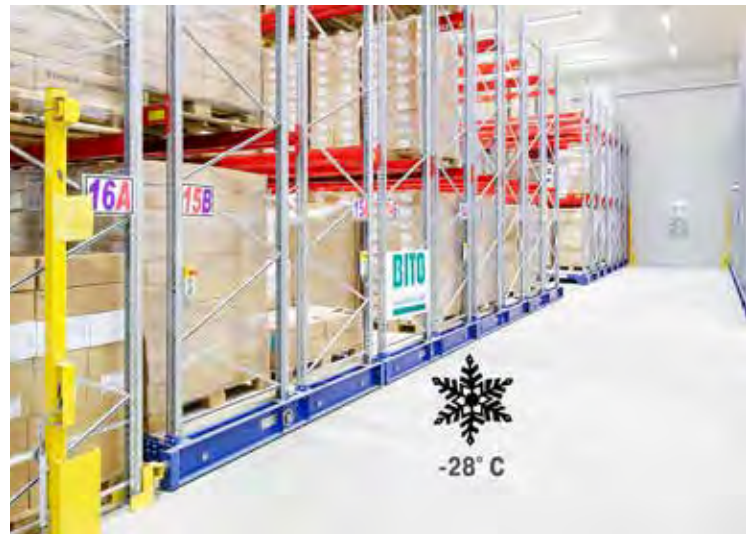
Mobile pallet racking in a cold store
