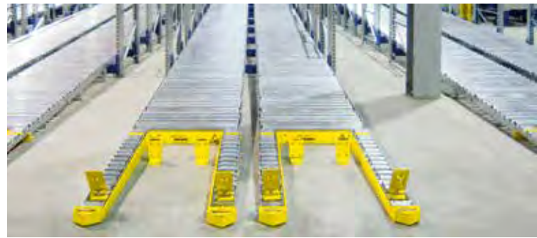
2-track segment for hand pallet truck retrieval
