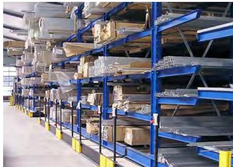
Mobile cantilever racking storing long loads
