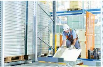
2. Open the door of the maintenance basket and place the starting board into the lane adjacent to the "trouble" lane.
