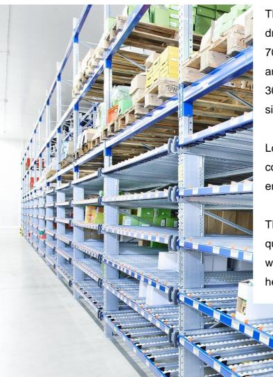
The use of carton live storage allows businesses to drastically cut down travel times (between 40% and 70%) compared with conventional shelving. The amount of floor space required is also reduced by up to 30%. These factors can save e-commerce retailers significant amounts of money.
