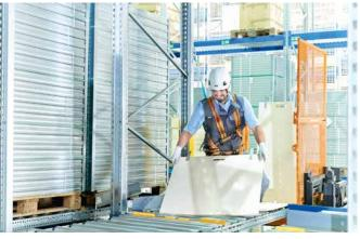
4. Push the intermediate board up to the yellow divider rail of the load separator.
