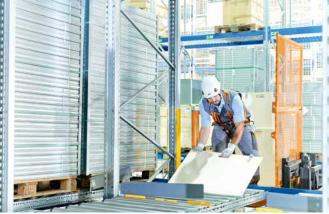
2. Open the door of the maintenance basket and place the starting board into the lane adjacent to the "trouble" lane.
