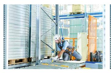
3. Swing activator of the FlowStop load separator to the side and secure it with the holding device.
