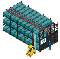
Operates according to the LIFO principle: last in, first out
