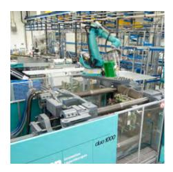
BITO bins and containers are produced in one of the most modern plants of the industry on high performance injection moulding machines with a clamping force of up to 27000 kN. After production, our bins and containers pass through our 600 sqm finishing centre where they are given the final touch to meet customer specific requirements. The entire manufacturing process combines high levels of automation with utmost versatility.
