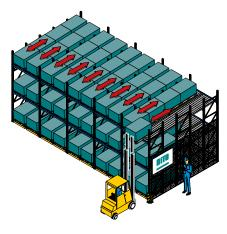
Operates according to the LIFO principle: last in, first out
