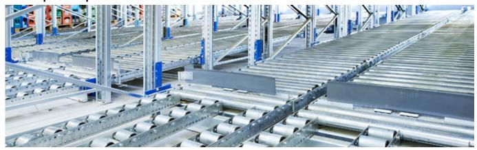
The BITO FlowStop load separator has been designed to reliably separate the first pallet at the picking face from the other pallets in the lane. This allows to retrieve the pallet at the picking face safely without lane pressure and without damaging the FlowStop load separator.
