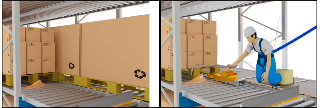
Figure 7: Removal of objects / packaging material in the lane.
