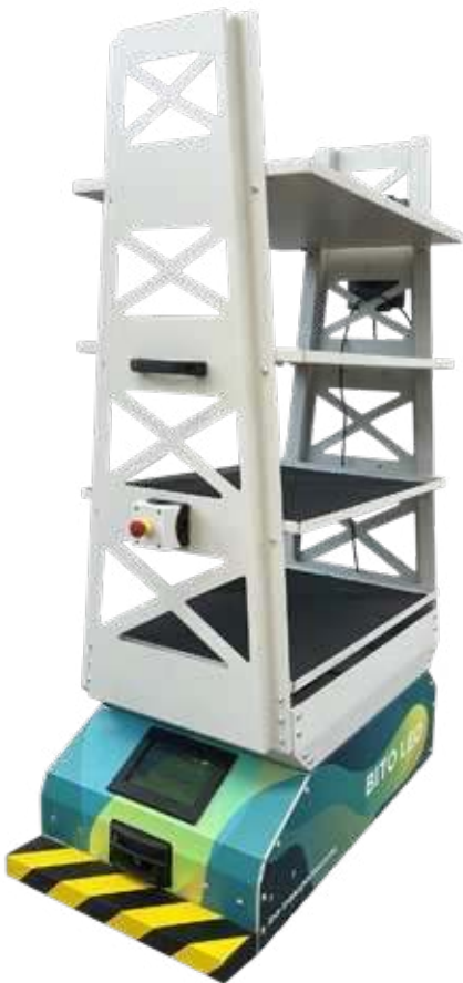
LEO carrier with on-top shelving and a mounted tablet for entering destinations
